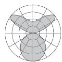
Direct Lumen Output: 429lm/ft Indirect Lumen Output: 509lm/ft CRI: 90+ (High Color Rendering)
