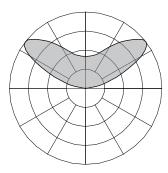
WB - LMO Wide Batwing (up to 139lm/W) Application: indirect wide spacing
