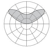
WB - LMO Wide Batwing (up to 139lm/W) Application: indirect wide spacing
