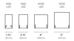
\*M-LED available in 1/4 in. increments. For Wet Location - restrictions apply.
