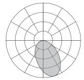
A2 - LMO Asymmetric 20° Wall Washer (up to 111lm/W) Application: wall washing
