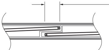
Lamps are spaced with 4" to 6" overlap to completely illuminate luminaire and eliminate socket shadows. Factory will supply approval drawings for other lengths using combinations of 21W & 28W T5 lamps or 39W & 54W T5HO lamps.
