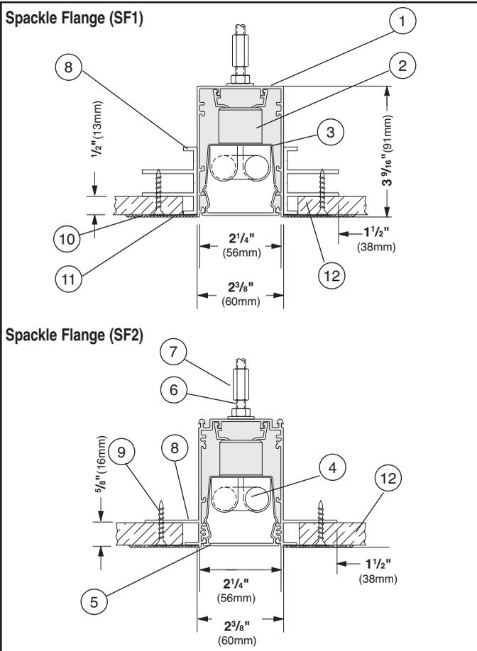
**1. Housing** - Continuous, 6063-T5 extruded aluminum profile up to 16 feet long. Joined with Connector Plus Joining System for ease of installation and to assure a uniform appearance.
