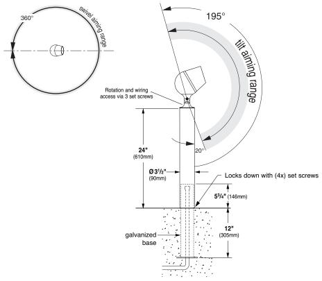
Concrete footing to be designed and installed by others.
